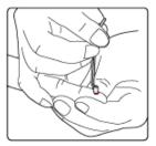
HOLD THE CAPILLARY TUBE HORIZONTALLY AND Collect the samples using capil lary action.
